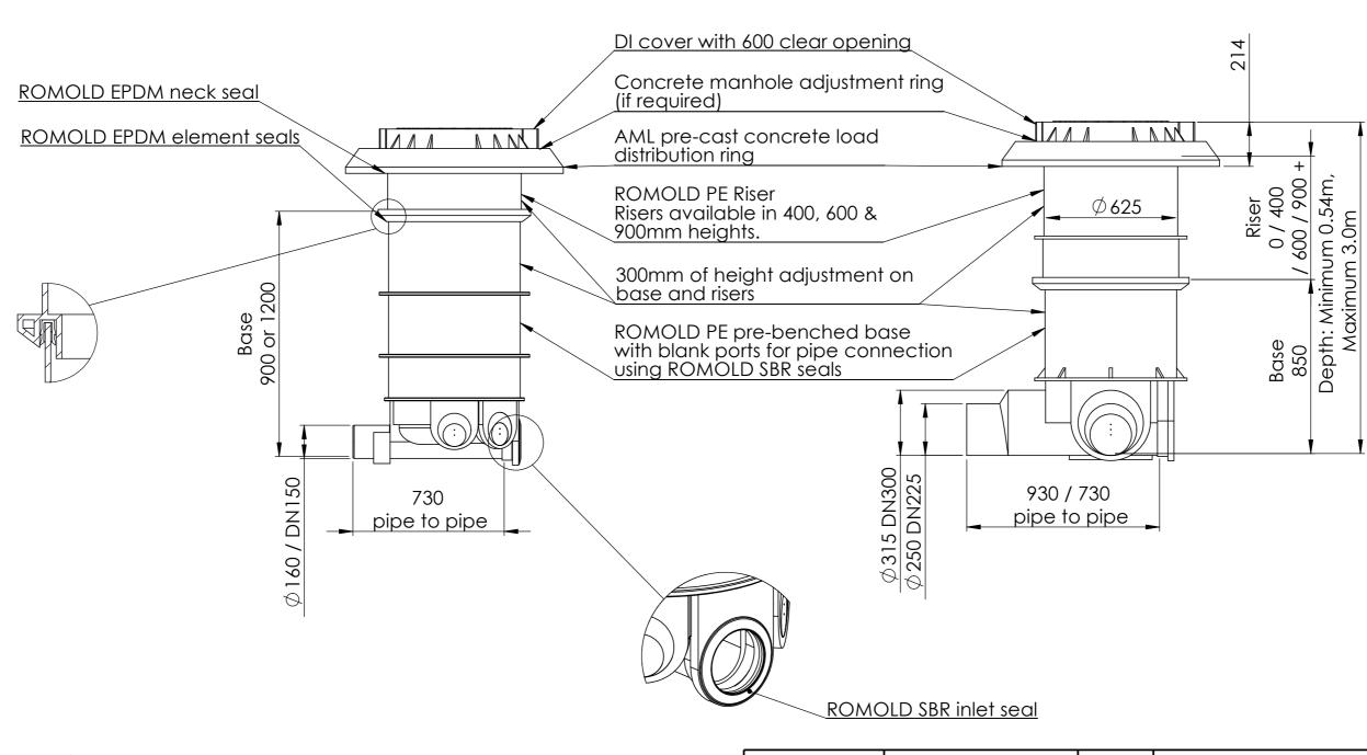
ROMOLD DN625 maintenance chambers are approved to EN 13598-2. Maximum depth to invert is 3m.
