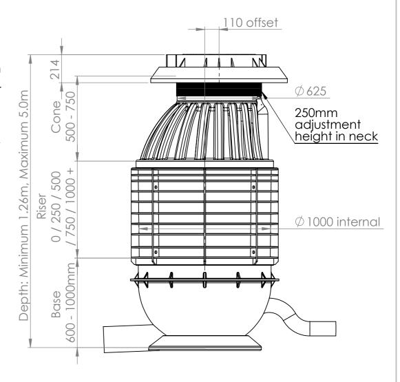
ROMOLD DN1000 manhole chambers for pressure sewer discharge. Maximum depth to invert is 5m. Maximum groundwater height is 4m. Suitable for Class D traffic loading (meeting HN-HO-72).
